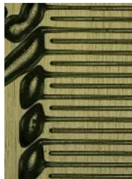
Etched IDE structure, line width 40 \mu m
